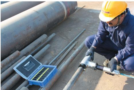
FM-3000 used during new boiler manufacturing and boiler maintenance.
